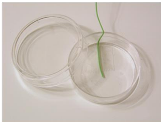
Figure 32. T Sensor secured inside a 35mm Petri Dish
