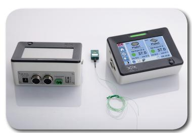
H601-NIKON-TI-SR-GLASS/FRAME must be connected to the user-friendly touch screen H401-T-CONTROLLER. This temperature controller offers two independent control channels, one for the optical glass and the other for the aluminum case.
