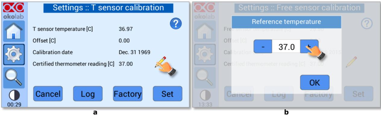
Figure 49. How to re-calibrate the T sensor
