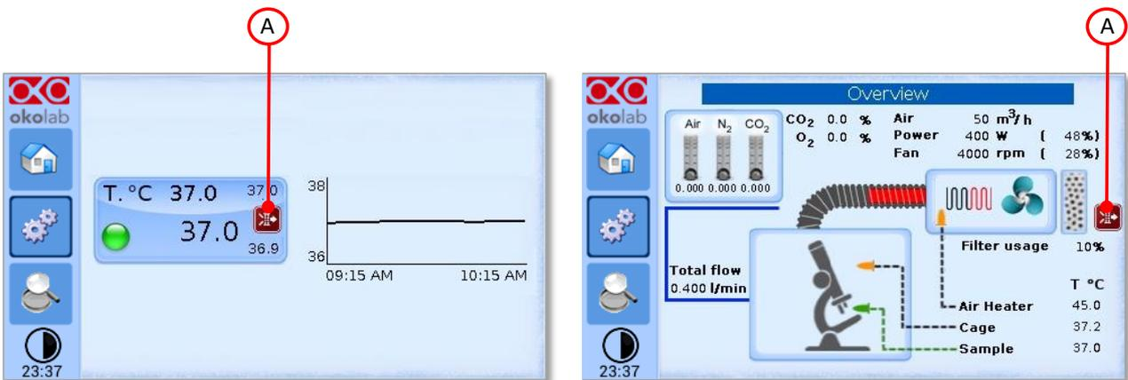
Figure 23. Home Page and Status Page when the usage time of the HEPA filter exceeds the maximum time of 360 days
