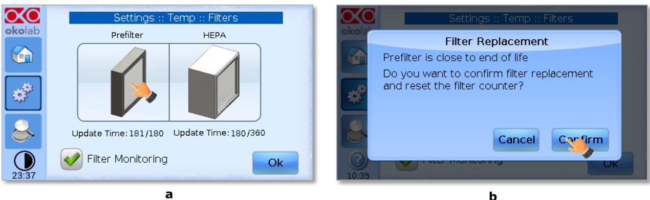
Figure 25. Warning for Prefilter replacement.
