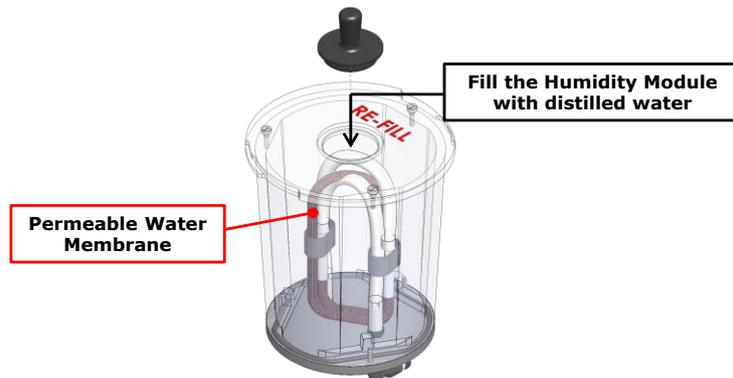
Figure 58. How to fill the Humidity Module.
