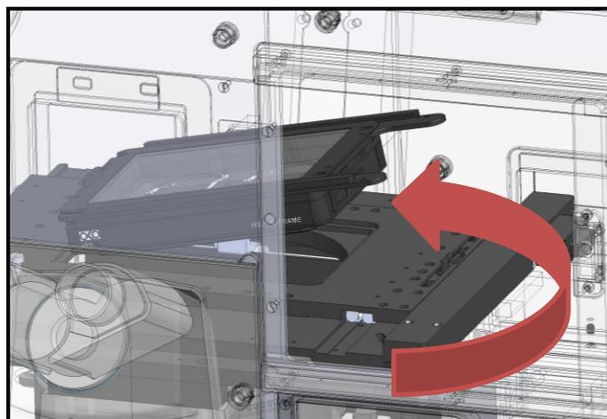
Figure 69. Chamber Incubator insertion inside the enclosure
