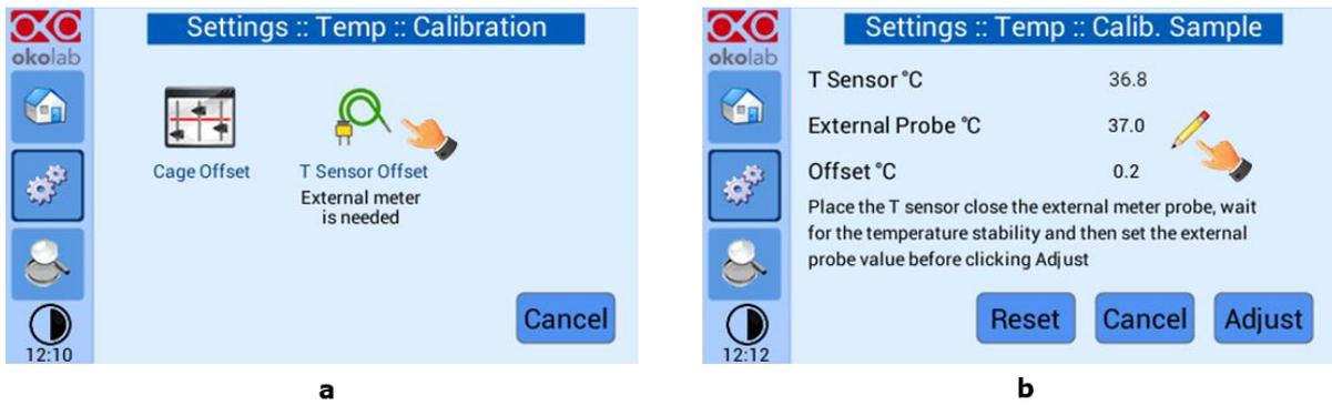
Figure 32. T sensor calibration (a-b)
