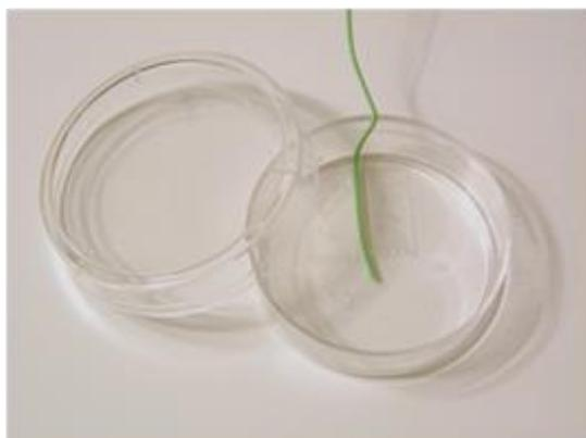
Figure 17. Free Sensor attached on the internal base of the Petri Dish
