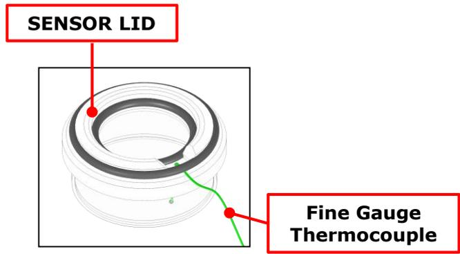
Figure 18. SENSOR LID-35. For 35 mm Petri-dish
