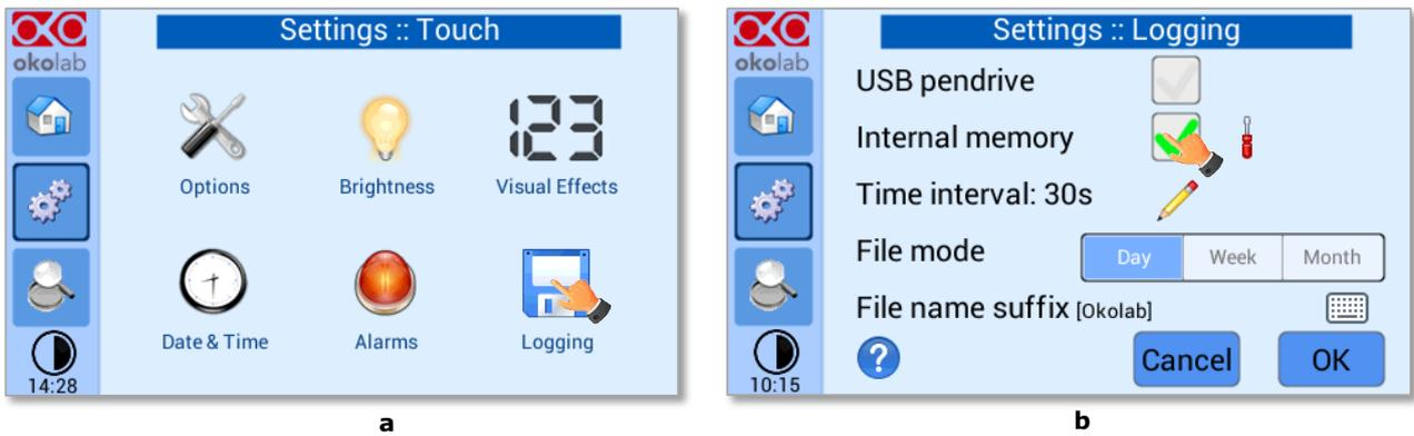
Figure 44. Logging. (a) How to enter in the logging menu; (b) logging in internal memory
