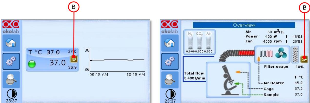
Figure 24. Home Page and Status Page when the usage time of the Prefilter exceeds the maximum time of 180 days
