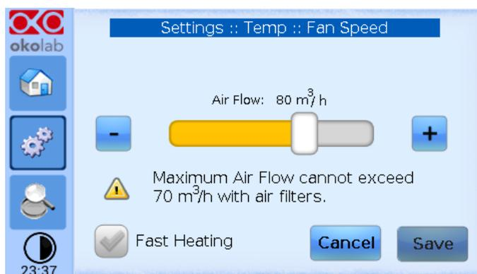
Figure 27. Air Flow Warning message when using Air Filters
