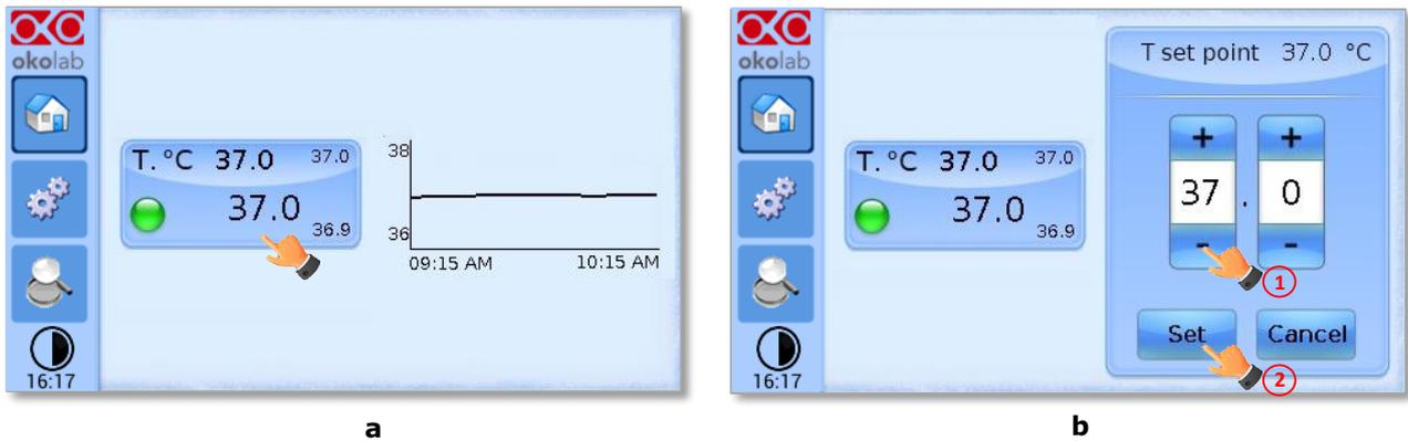
Figure 10. How to change the Temperature set point (a - b)
