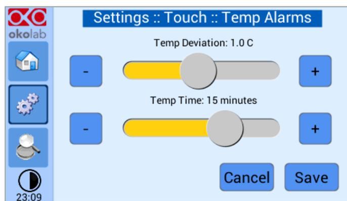
Figure 41. How to set the Deviation and Time Alarm
